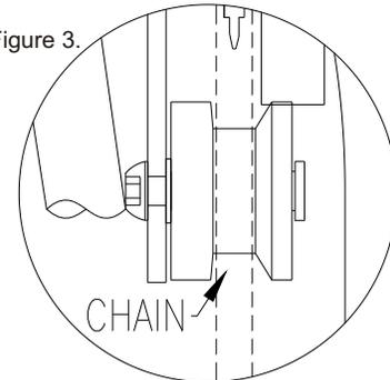
13. When everything is installed correctly, **SPACING A**(**Figure 2.**) should be between **4mm & 6mm**, and the groove of the **ROLLER** should be inline with the middle chainring as show in **FIGURE 3**. The **CHAIN** should ride in the groove of the **ROLLER** when it is on the middle chainring and when you shift to the granny chainring the chain should shift up onto the tall step of the **ROLLER**.
