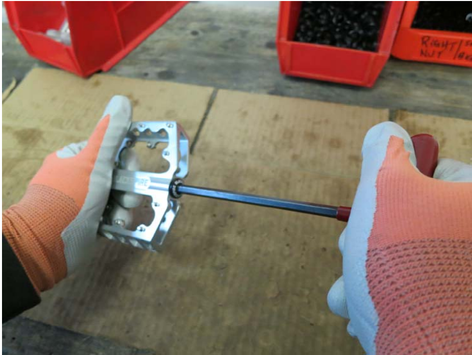
Figure 1: Holding the pedal body with a hand and removing the endcap with the 6 mm hex key wrench.
