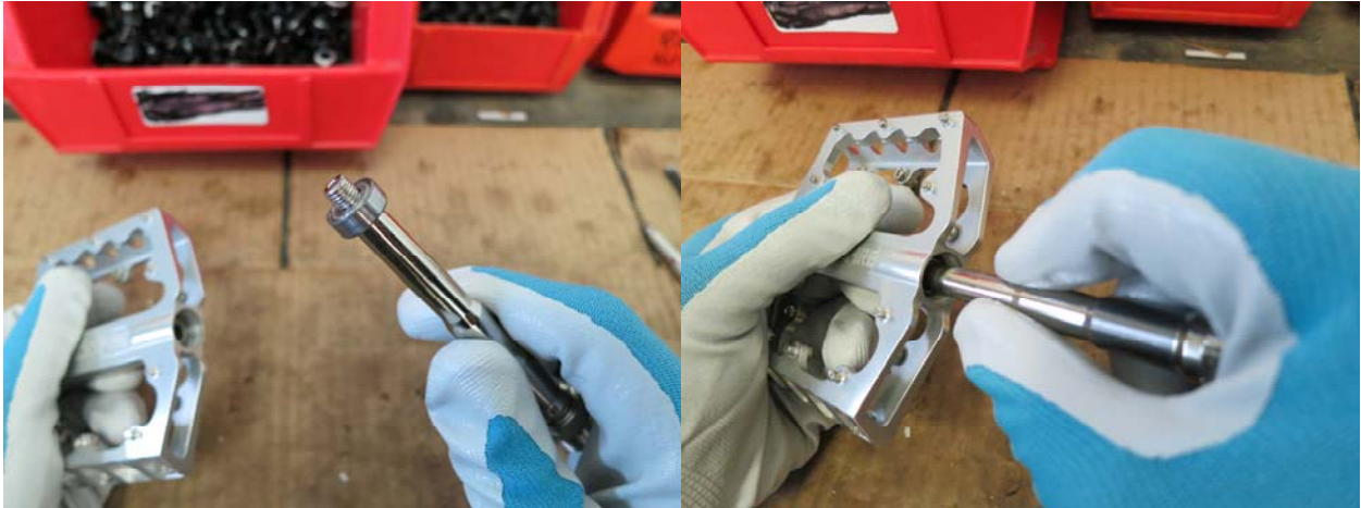
Figure 5: The 686 bearing is placed onto the pedal axle (left) and inserted into the pedal body (right).
