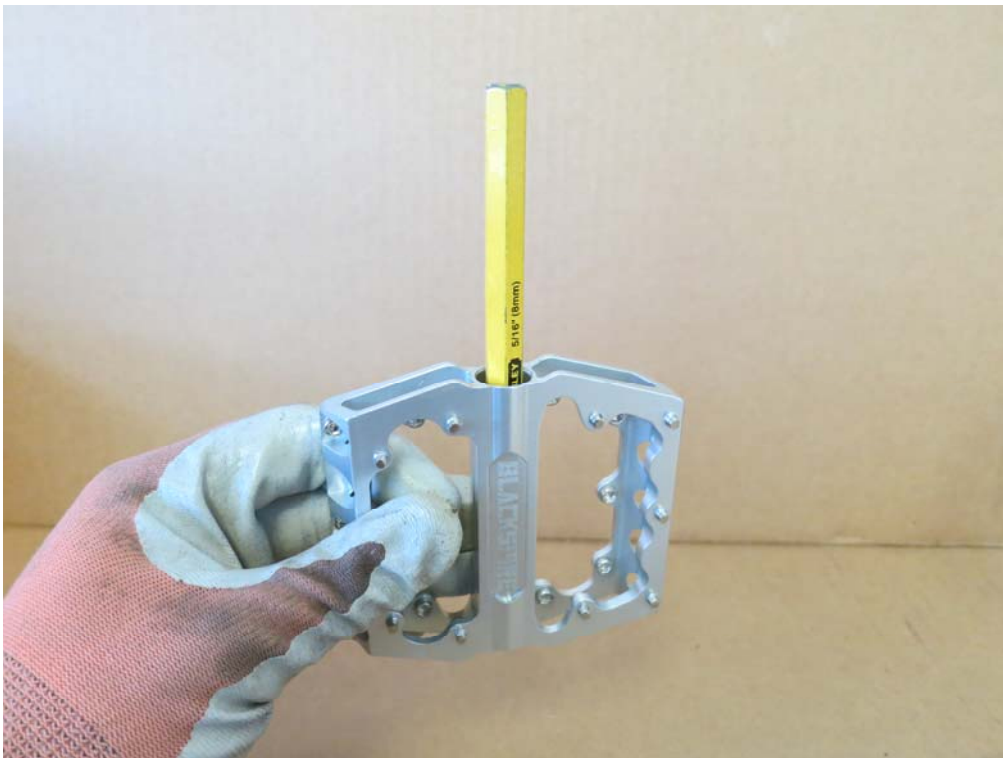
Figure 4: Insert the 6 mm or 8 mm tool punch through the bushing side and gently tap it to push out the 686 bearing.
