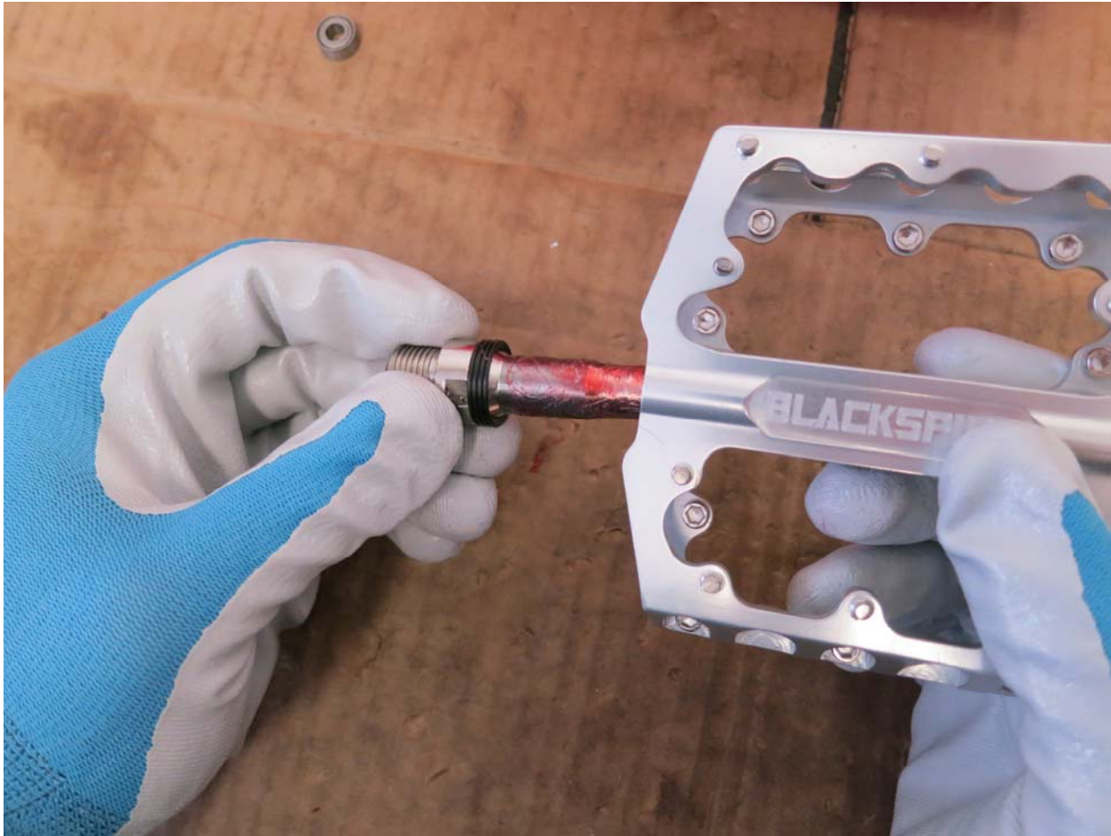
Figure 7: Inserting the greased pedal axle into the pedal body.
