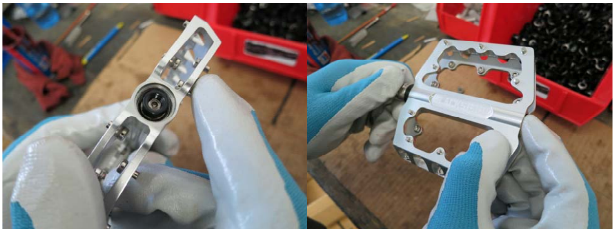
Figure 8: Applying (left) and tightening (right) the pedal axle nut by turning the pedal axle until it is hand tight.
