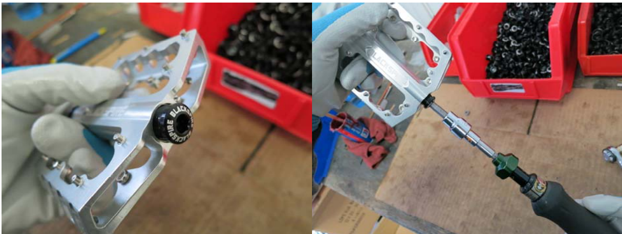
Figure 10: Tightening the end cap onto the pedal body to the torque specification of 4 Nm.
