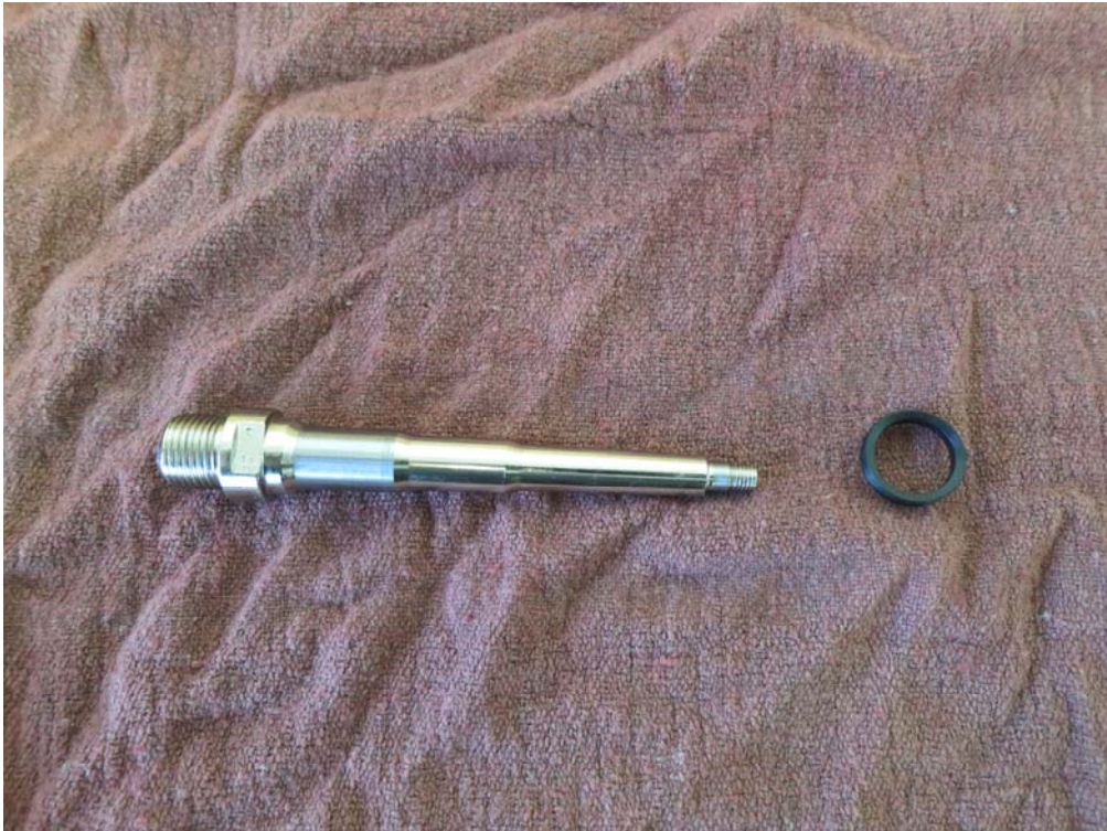
Figure 3: Cleaned pedal axle with the seal removed.
