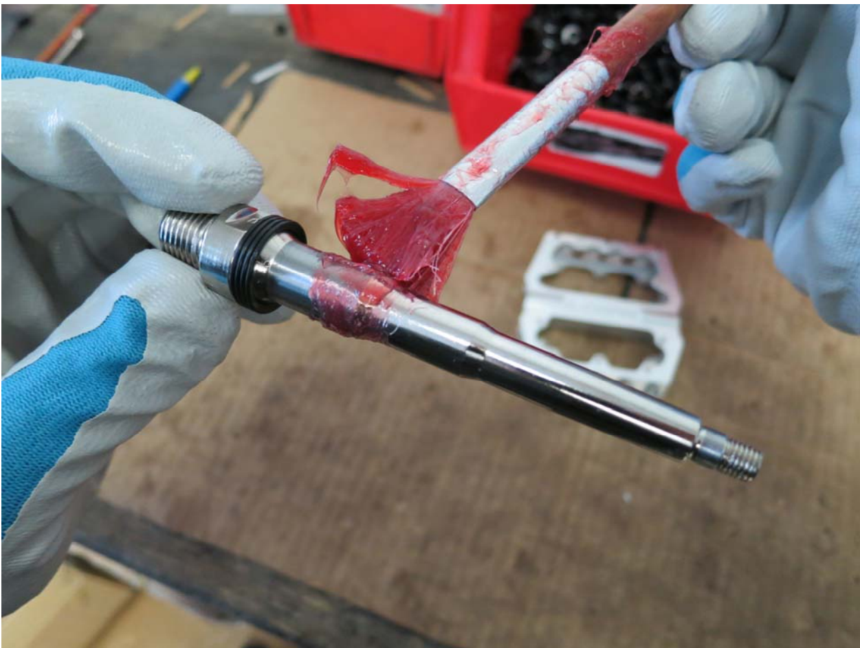
Figure 6: Applying grease onto the split DU bushing seat on the pedal axle. Notice the final location of the rubber seal.
