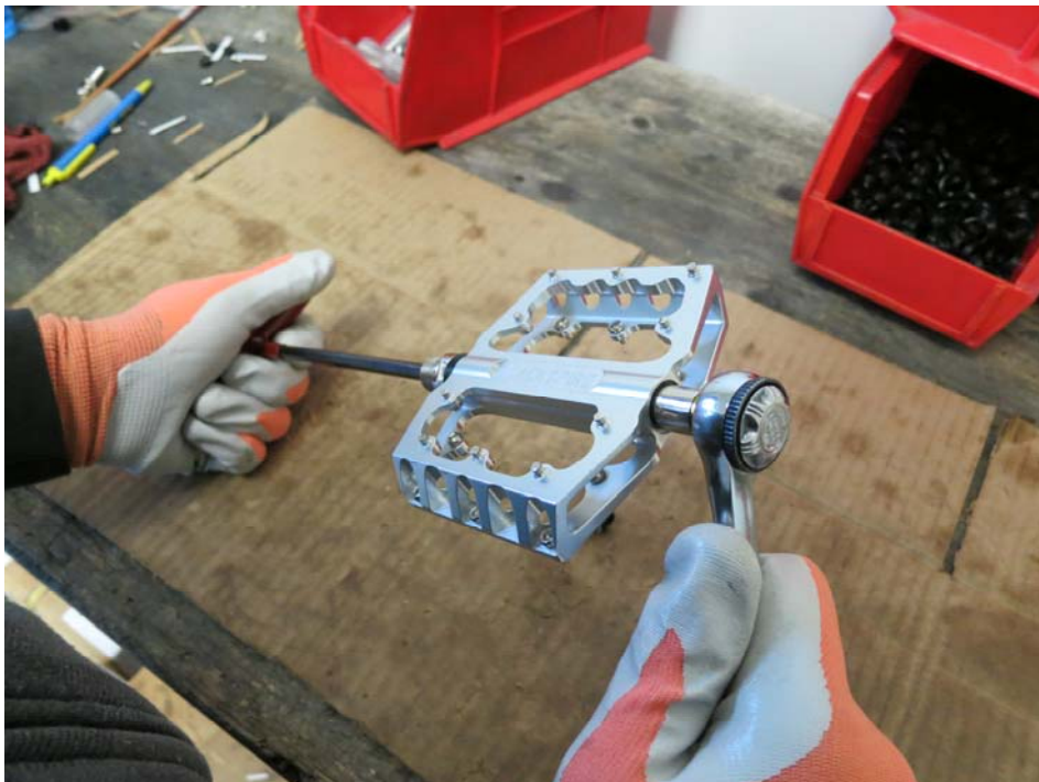
Figure 2: Holding the pedal axle stationary with the 6 mm hex key wrench and loosening the pedal axle nut with the 9 mm 6-point socket.
