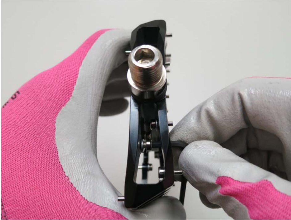
Figure 5: Tightening the traction pin with traction pin spacer into the pedal body using the flat tipped 3 mm hex key wrench.
