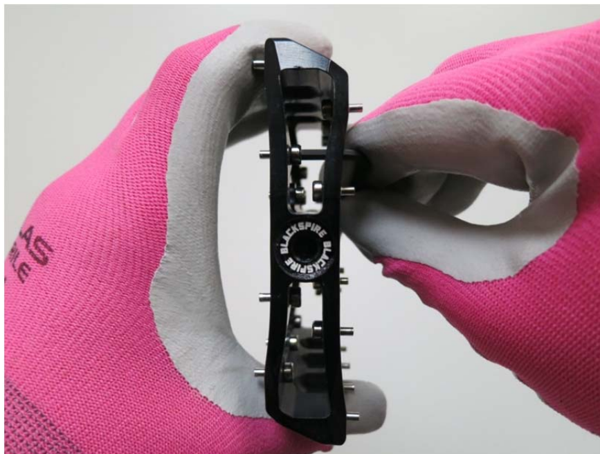
Figure 2: Loosening the traction pins from the pedal bodies using the flat tipped 3 mm hex key wrench.
