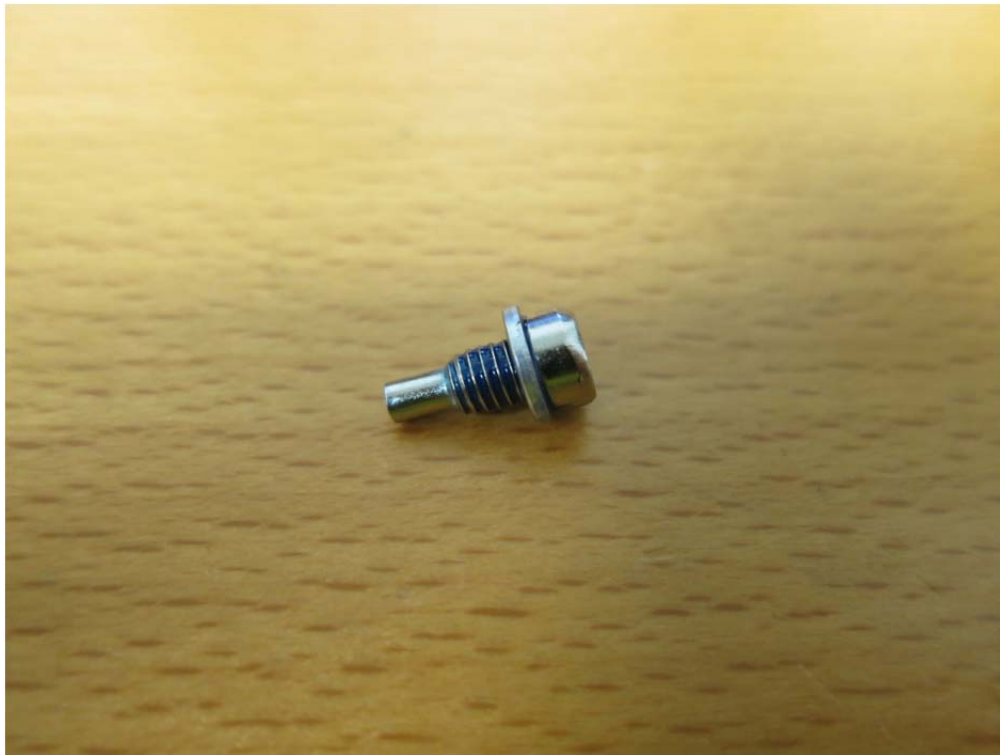
Figure 4: Loctite applied on the threads of the traction pin.
