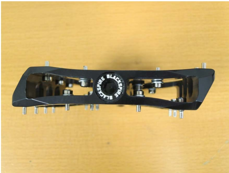
Figure 6: Final traction pin height configuration may differ from the one depicted above depending on rider's preference.
